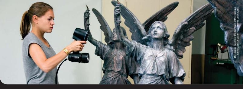
Creaform presents Go!SCAN 3D™, a **simple**, portable and affordable **3D scanner** allowing people from various backgrounds to effortlessly capture the 3D shape of any object, including complex, freeform and organic shapes. The resulting 3D models can then be used in all of your computer-assisted processes: archiving, restoration, analysis, content creation...
