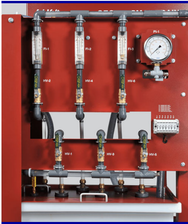
Ground loop header.
