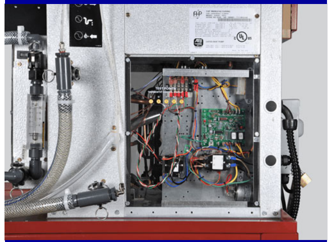
Connections to the control board are provided for troubleshooting purposes.
