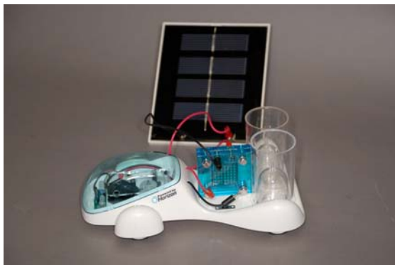
Fuel-Cell used to power a car
