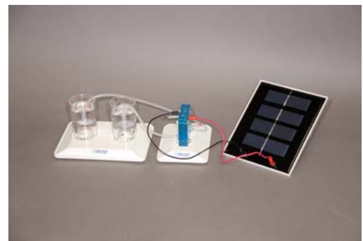
Fuel-Cell charged by a 1-W Solar Panel
