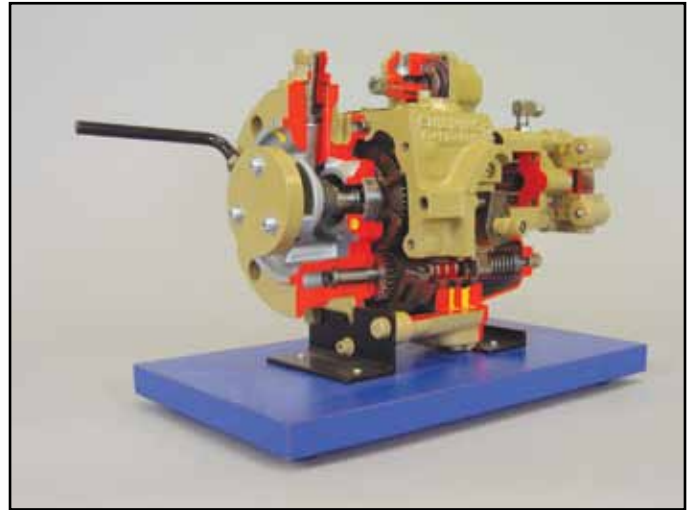
PT Cummins Diesel Injector Pump Model 6682
