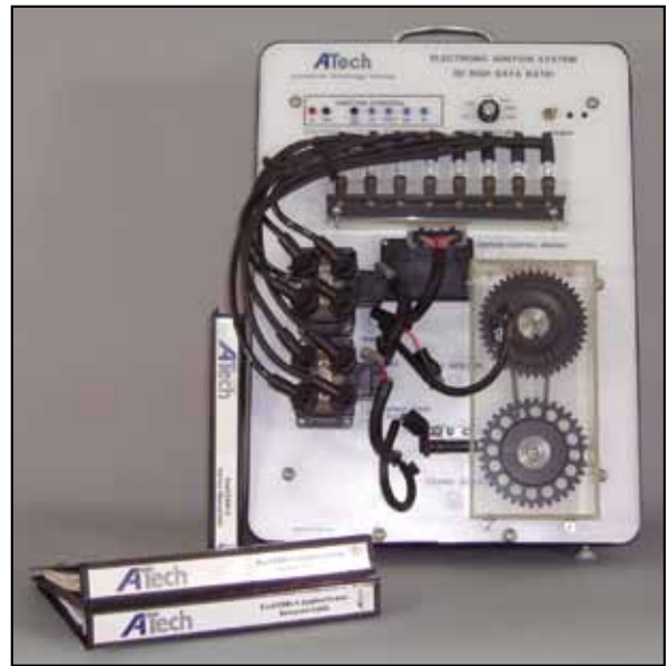
Ford EDIS-V Ignition System Model 1791F
