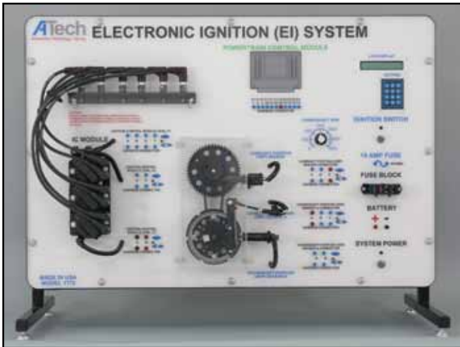
GM Electronic Ignition (EI) System Model 1772
