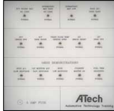
EEC-V System Fault Panel
