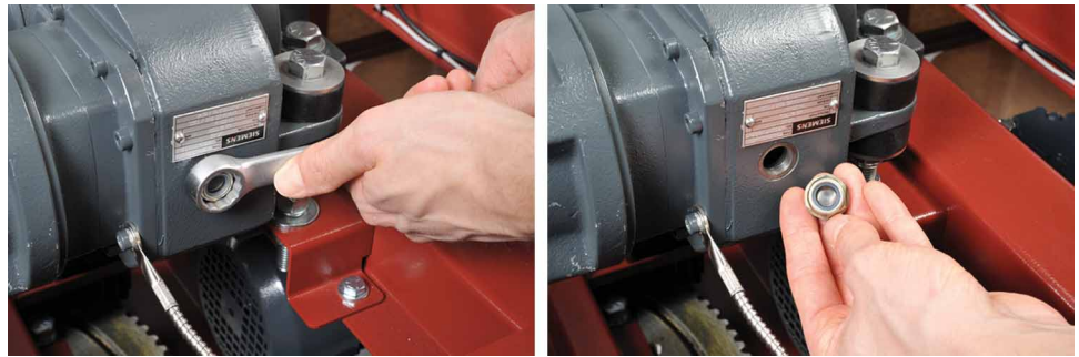
Figure 2-55. Removing the sight glass plug.
