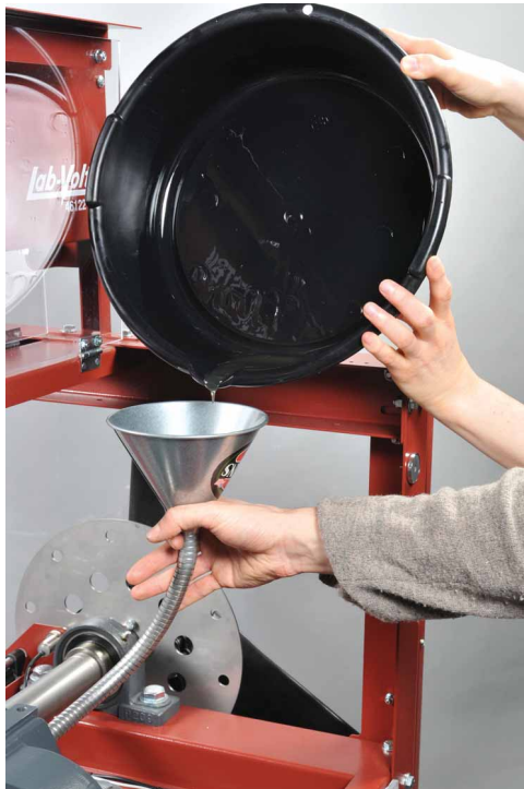
Figure 2-56. Pouring new oil into the gearbox.
