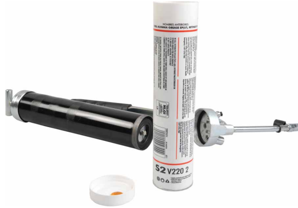
Figure 2-41. Removing the plastic cap.
