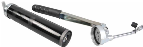
Figure 2-40. Opening the grease gun.
