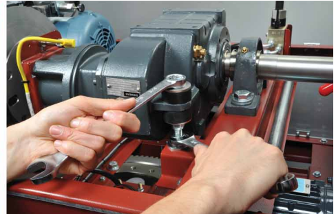
(b) second nut rotation (bolt remains static)
