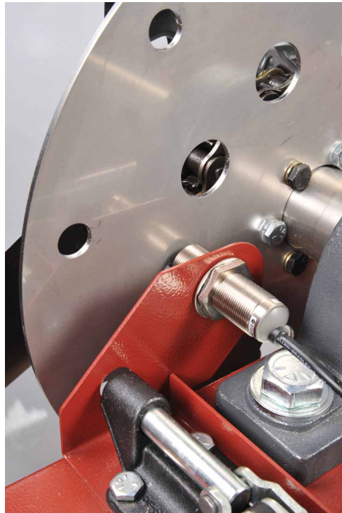
Figure 2-23. Inductive sensor and perforated disc.
