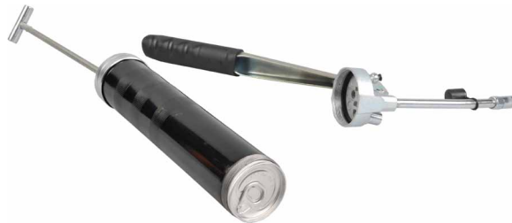
Figure 2-42. Inserting a new grease cartridge.
