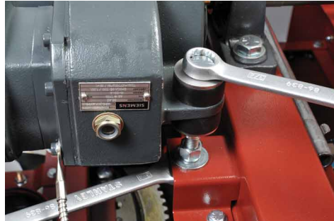
(a) bottom nut rotation (bolt remains static)
